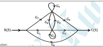
For the signal flow graph shown in below Fig., determine C/R using mason's gain formula.
